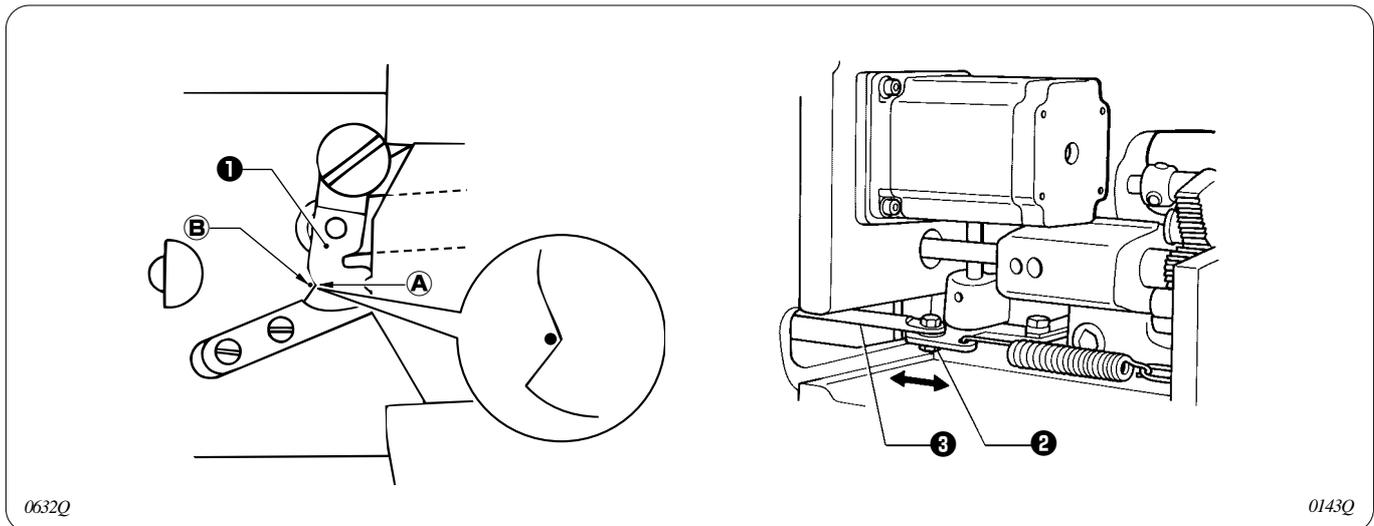
Loosen the nut **2** and move the connecting rod lever **3** to the left or right to adjust so that the V section **A** is aligned with the index mark **B** on the needle plate when the sewing machine in the stopped position and the movable knife **1** is pushed to the machine pulley side so that there is no play.
