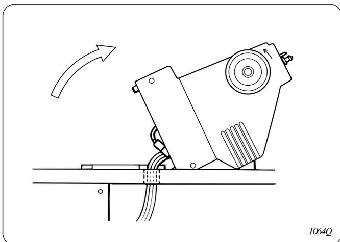
Gently tilt back the machine head with the belt cover attached in the direction of the arrow.
