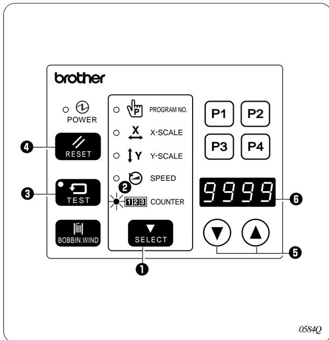
1. Press the SELECT switch **1** until the COUNTER indicator **2** illuminates.
