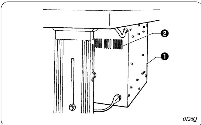
Use a vacuum cleaner to clean the filter in the air inlet port **2** of the control box **1** at least once a month.
