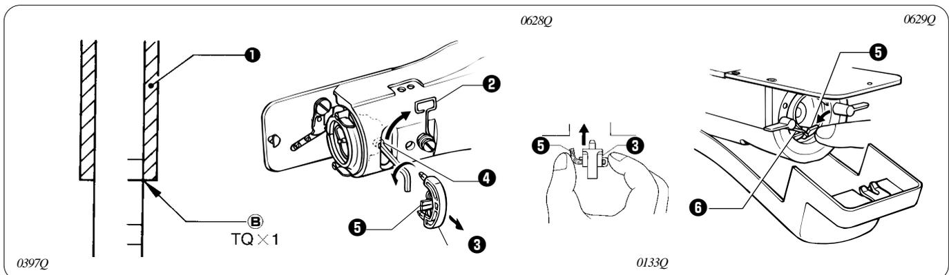
Adjust the needle bar lift amount as described below so that the tip of the rotary hook is aligned with the center of the needle when the machine pulley is turned to raise the needle bar from its lowest position until the second reference line from the top of the needle (reference line **B**) is aligned with the lower edge of the needle bar bush **1**.
