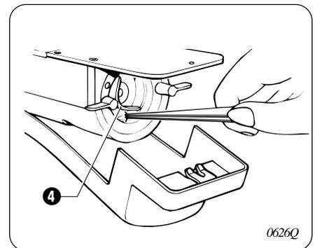
3. Clean all the dust and thread ends from around the driver **4**, the top of the rotary hook thread guide and the shuttle race.
