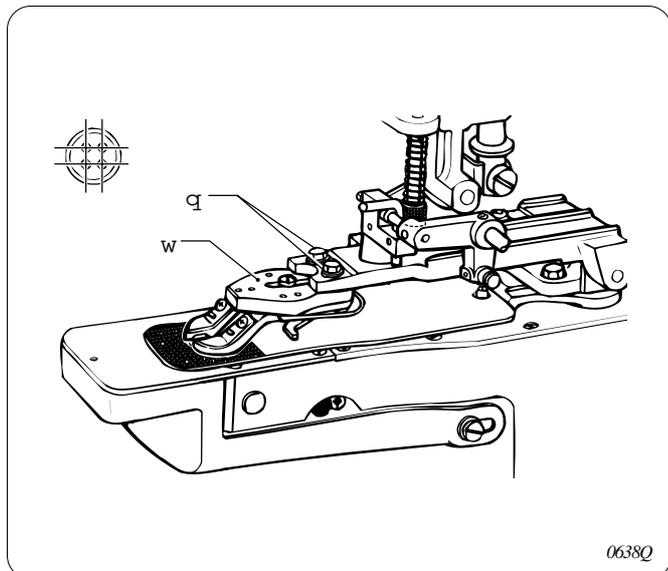
1. Loosen the two hexagonal bolts **1** and adjust the button holder body **2** by moving it.
