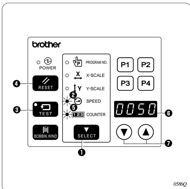
1. Press the SELECT switch **1** until the SPEED indicator **2** illuminates.
