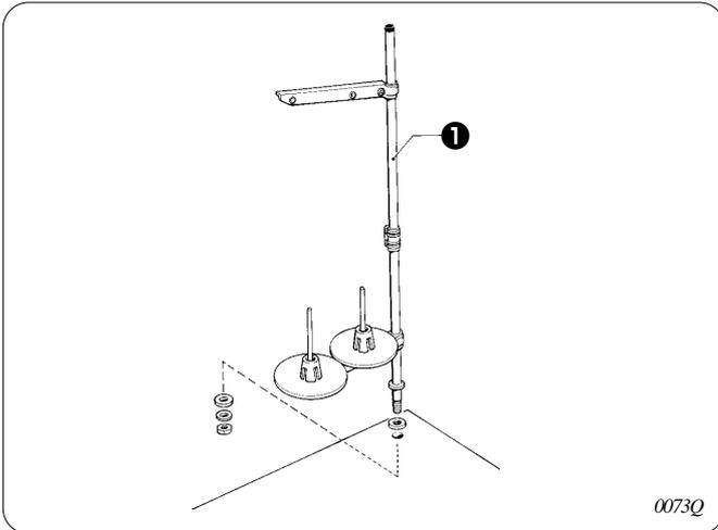
Assemble the spool stand **1** while referring to the spool stand instruction manual, and then install the spool stand **1** at the right side of the work table.
