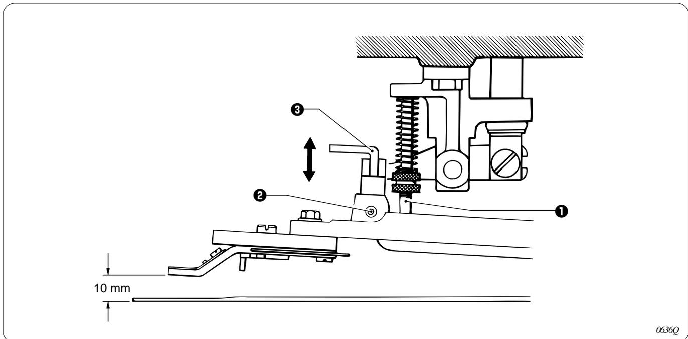
The button clamp lift amount is 10 mm from the top of the needle plate.
