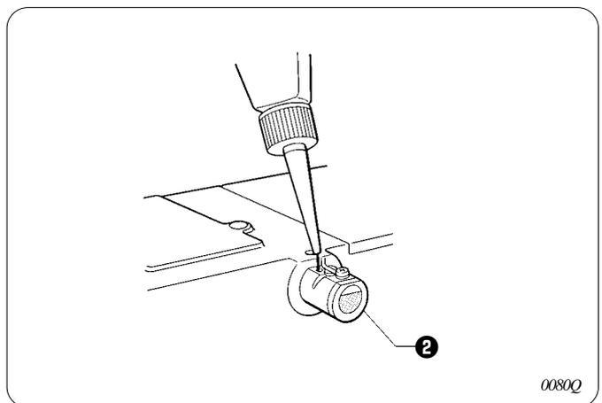
4. If using the liquid cooling tank ②, fill it with silicon oil (100 mm<sup>2</sup>/s).
