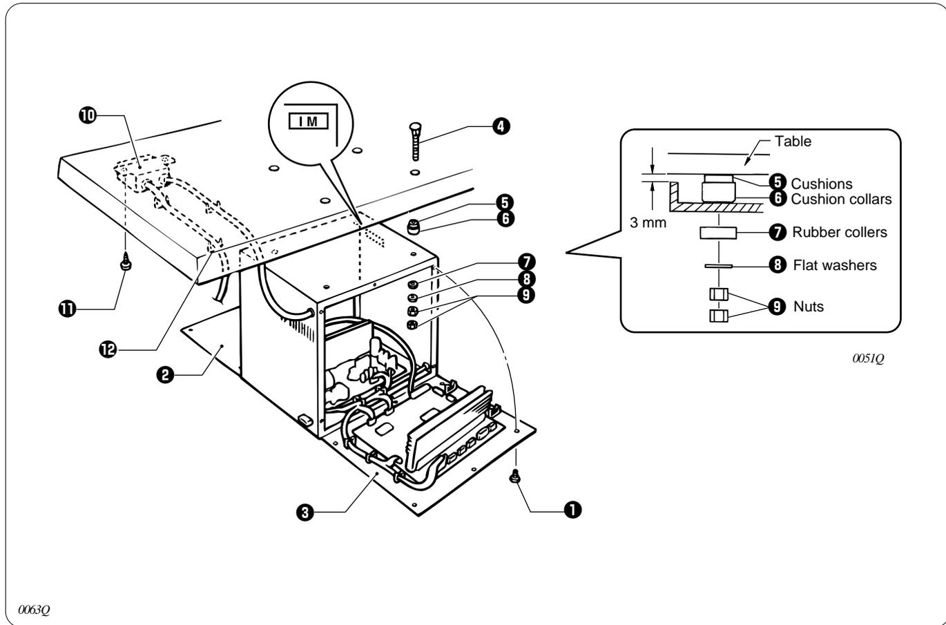
1. Remove the 12 screws **1**, and then open the covers (panel mounting assembly **2** and main P.C. board mounting plate **3**).
