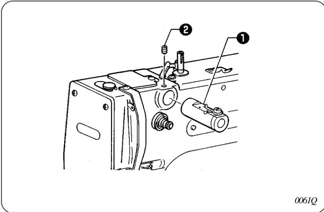
1. Remove the rubber plug, and then push the liquid cooling tank **1**.
