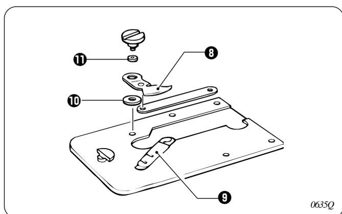
4. Remove the movable knife **8** and replace it with a new one. At this time, check that the movable knife **8** and the fixed knife **9** cut the thread cleanly. If necessary, adjust by using the appropriate movable knife washer **10** (supplied as accessories).
