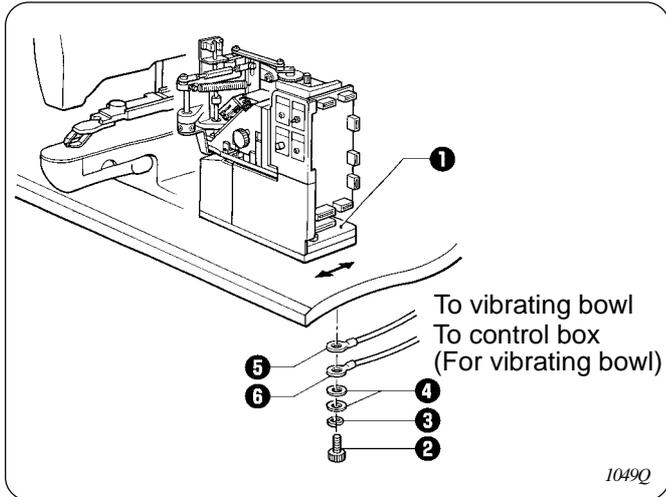
1. Move button feeder base **1** to the front and rear and left and right as necessary to install it by using hole bolts **2**, spring washers **3** and washers **4**. (And install ground wires **5** **6**.)
