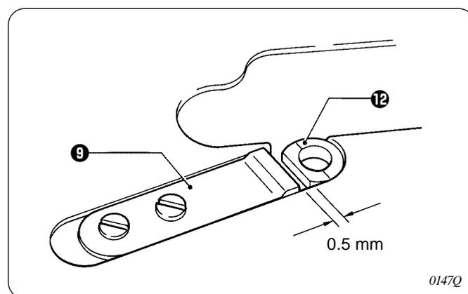
5. Install the fixed knife **9** at a distance of 0.5 mm from the needle hole plate **12**.
