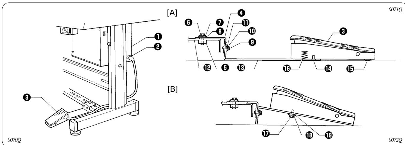
1. Insert the connector of the foot switch **3** into the connector **2** of the control box **1**.
