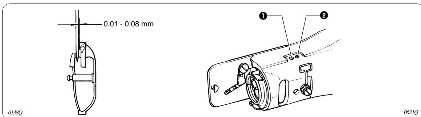
Turn the machine pulley to align the tip of the rotary hook with the needle center line. Then loosen the set screw **1** and turn the eccentric shaft **2** to adjust so that the clearance between the needle and the rotary hook is 0.01 - 0.08 mm.
