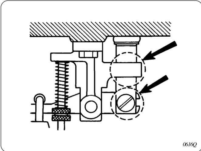
Do not apply too much grease in the place indicated by the arrow. If too much grease is applied here, the button clamp may not move up and down smoothly and error [E-6□] may appear on the display.
