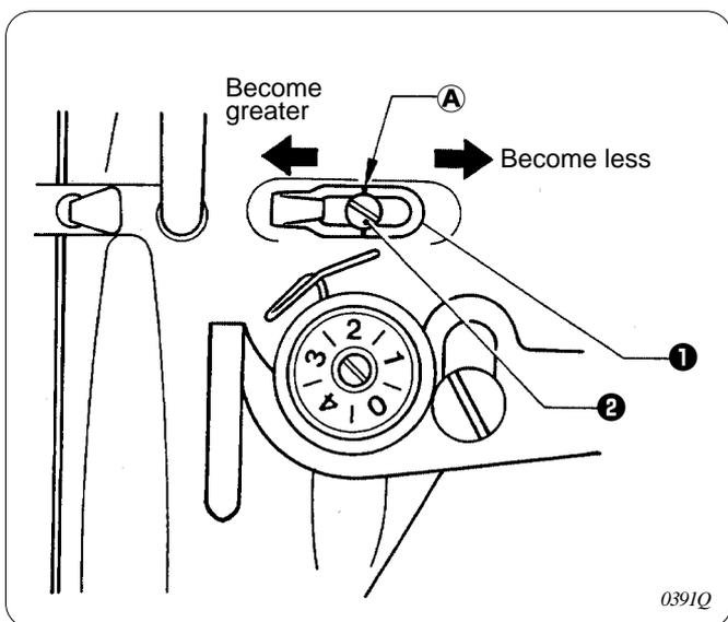
The standard position of arm thread guide R ❶ is when the screw ❷ is aligned with mark A.
