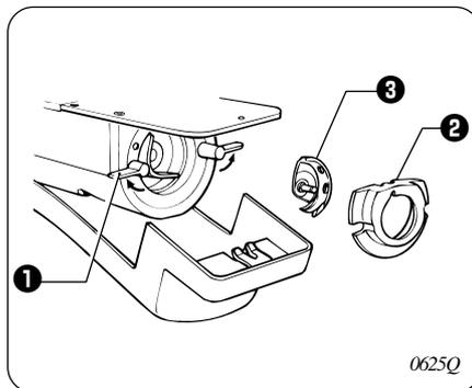
2. Open the setting claw **1** in the direction indicated by the arrow, and then remove the shuttle race body **2** and the shuttle hook **3**.
