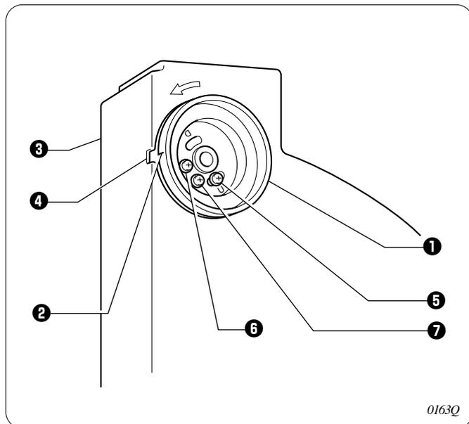
The needle up stop position is adjusted so that the index mark **2** on the machine pulley **1** is inside the mark **4** on the belt cover **3**.
