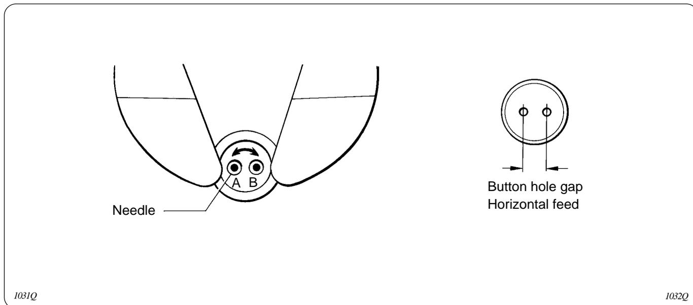
1. Set the X scale so that the holes A and B in the button are aligned with the point of the needle. (Refer to "Setting the X-scale and Y-scale" on page 23.)
