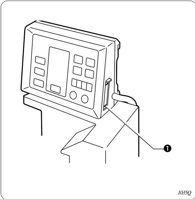
The operation panel DIP switches ① are used to change functions which might need to be changed depending on the sewing conditions.
