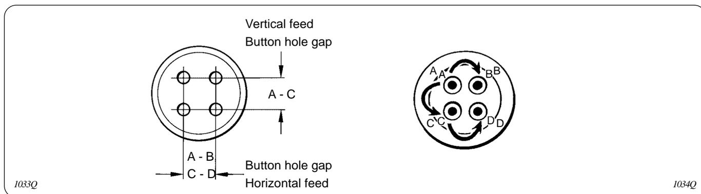
1. Set the Y scale so that the holes A and C in the button are aligned with the point of the needle. (Refer to "Setting the X-scale and Y-scale" on page 23.)
