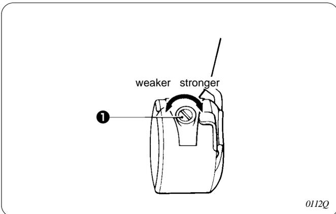
Adjust the thread tension to the weakest possible tension by turning the thread tension nut **1** until the bobbin case will not drop by its own weight while the thread end coming out of the bobbin case is held.
