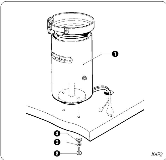
1. Install the vibration bowl **1** with bolts **2**, spring washers **3**, and washers **4**.
