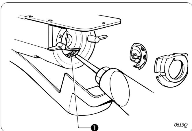
3. Add oil to the felt ① of the shuttle race base.
