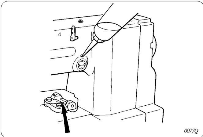
1. Fill the arm-side oil tank with oil.
