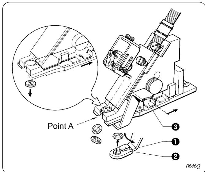
1. Turn the button carrier **1** by hand in the direction of the arrow, and remove any buttons from the button carrier pin **2**.
