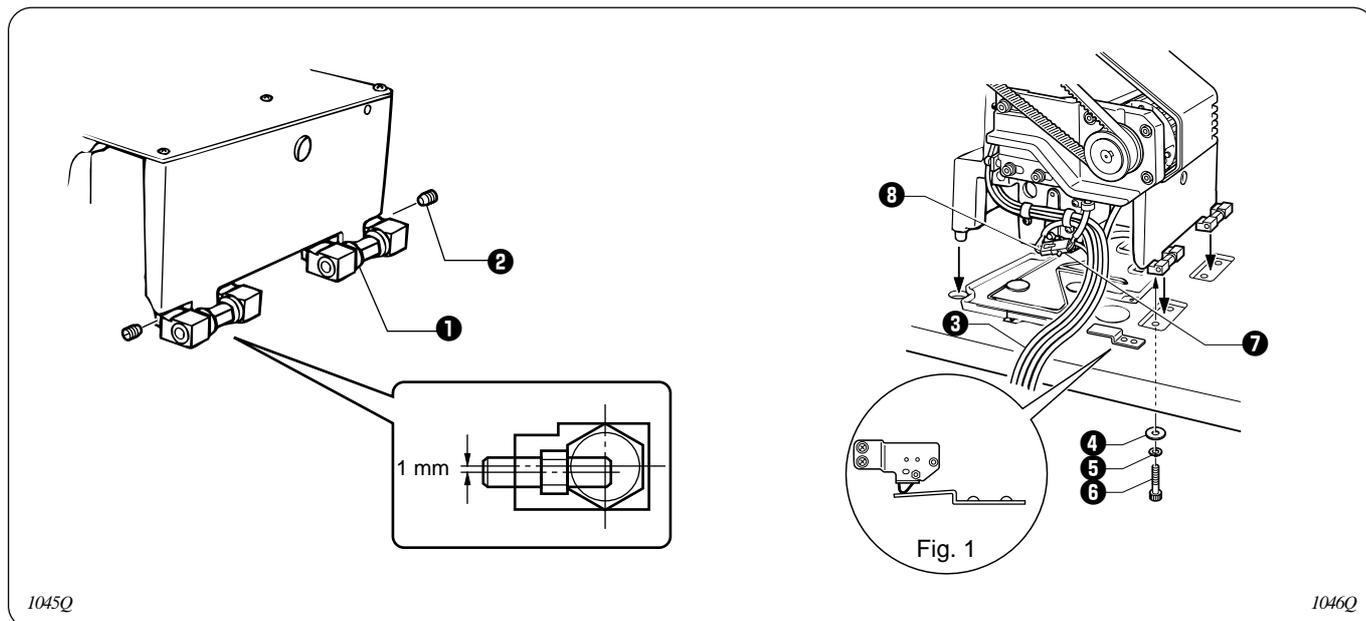
1. Insert the two hinge assemblies **1** into the machine head so that they are parallel, and then secure them with the two set screw **2**.
