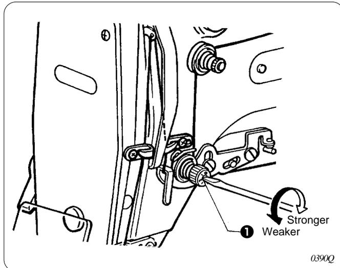
Turn the tension stud ❶ with a screwdriver.
