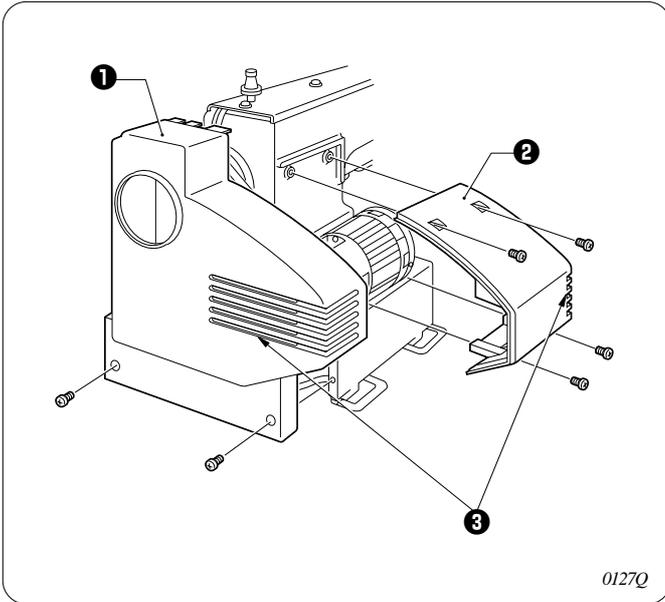
Remove the belt cover ① and the frame side cover ②, and then clean the air holes ③. After cleaning, install the belt cover ① and the frame side cover ②.
