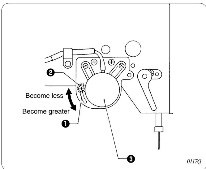
Loosen the screw ❶ and move the stopper (3.57 nut) ❷ to adjust the operating angle of the thread take-up sole-noid ❸.
