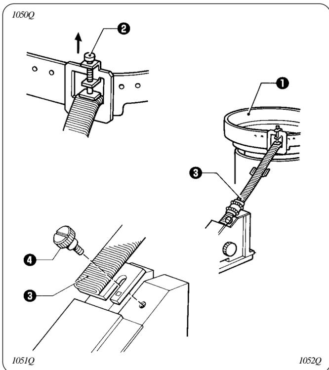
1. Raise the shooter lock pin **2** on the vibrating bowl **1**, and secure the shooter **3** by inserting the pin **2**, through the notch in the shooter.
