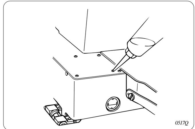
2. Fill the bed-side oil tank with oil
