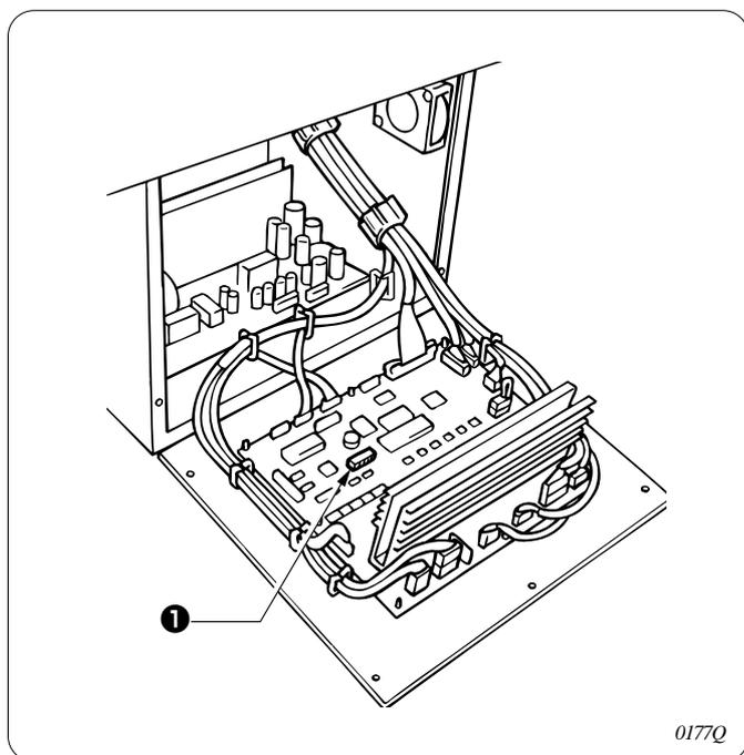
The DIP switches ❶ inside the control box are used to change functions which do not often need to be changed once they have been set.
