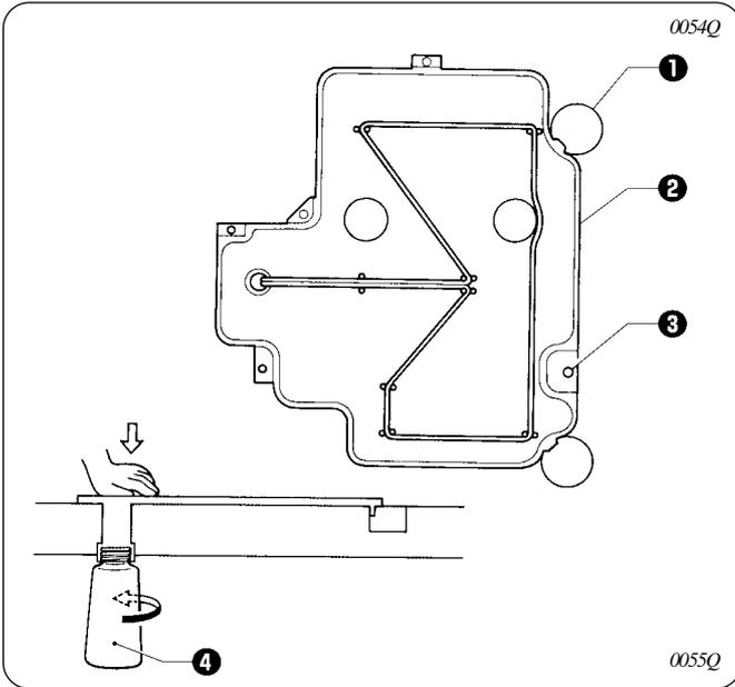
1. Insert the tabs of the oil pan **2** into the holes for the cushions **1**, and then secure it in place with the five nails **3** so that the oil pan **2** is not at an angle.
