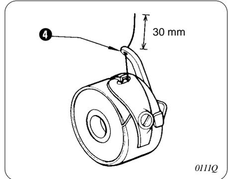
Pass the thread through the lever thread hole **4**, and then pull out approximately 30 mm of thread.
