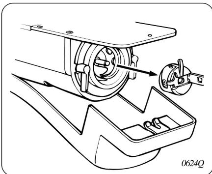
1. Pull the shuttle race cover toward you to open it, and then remove the bobbin case.
