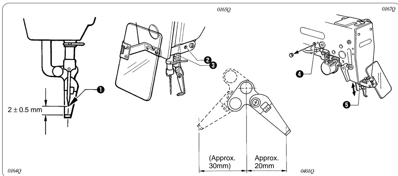
1. Loosen the set screw **2** and move the wiper arm support **3** up or down to adjust so that the clearance between the top of the thread wiper and the needle point **1** is  $2 \pm 0.5$  mm when the thread wiper is aligned with the center of the needle.
