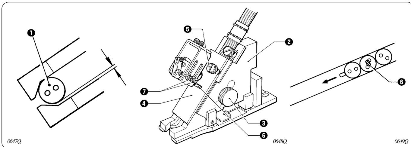
1. Adjust the width of the slide base assembly **2** to the button width with slide base screw **3** so that the buttons **1** pass smoothly.
