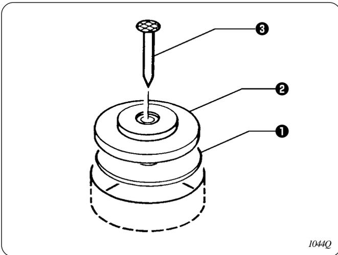
1. Place the washers **1** and cushions **2** into the two holes in the work table.
