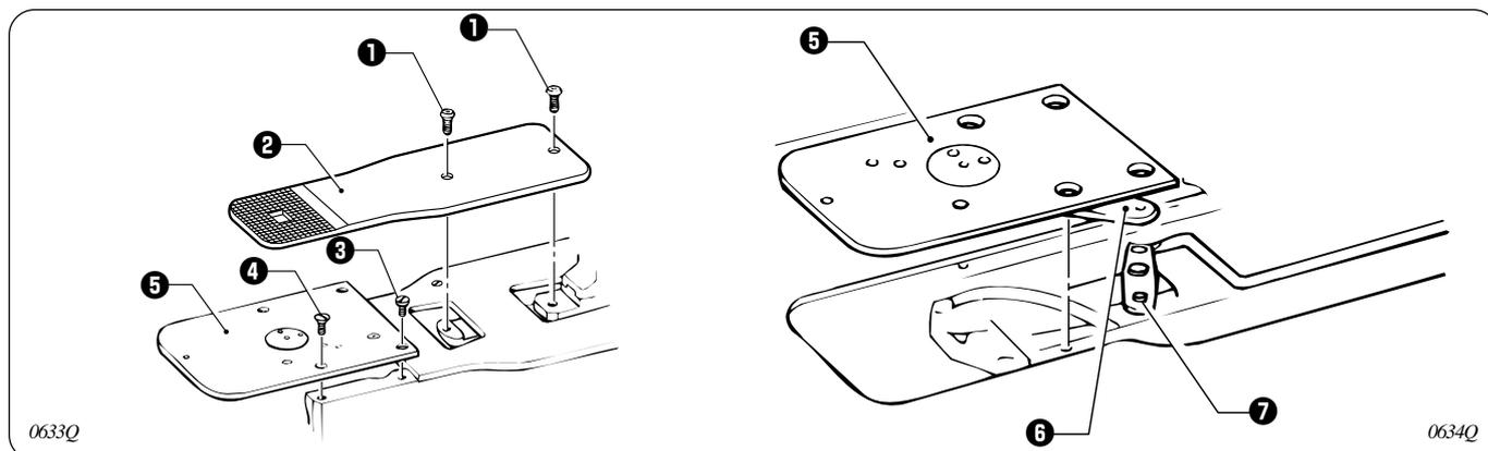
1. Open the large shuttle hook cover, remove the screw **1**, and then remove the feed plate **2**.
