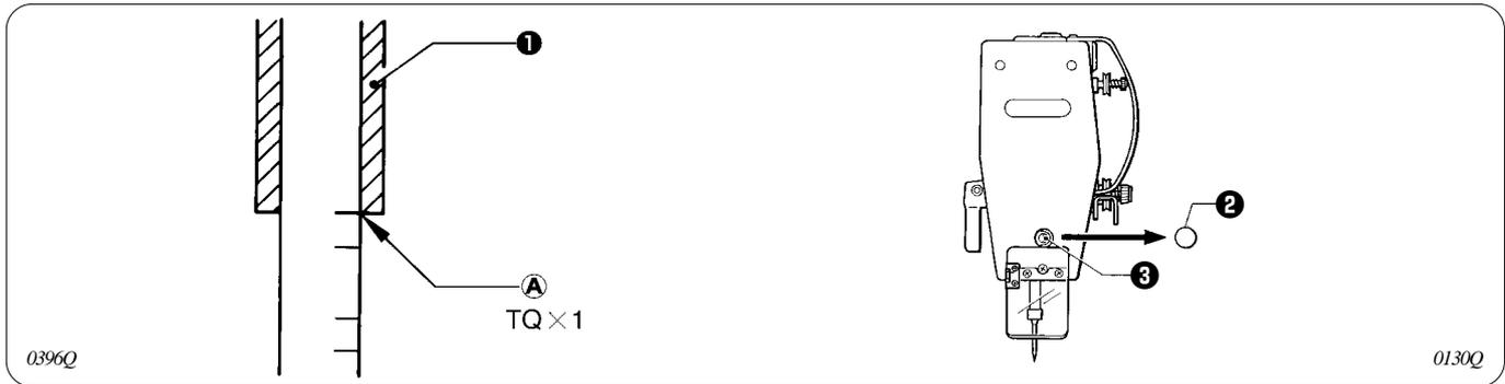
Turn the machine pulley to move the needle bar to the lowest position. Then remove the rubber plug **2**, loosen the set screw **3** and then move the needle bar up or down to adjust so that the highest reference line (reference line **A**) is aligned with the lower edge of the needle bar bush **1**.
