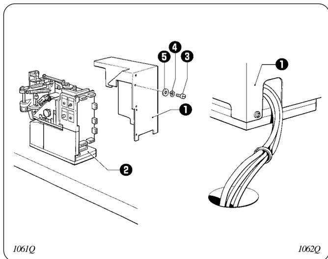
Attach the button feeder cover **1** to the button feeder **2** with screws **3**, spring washers **4**, and washers **5**.
