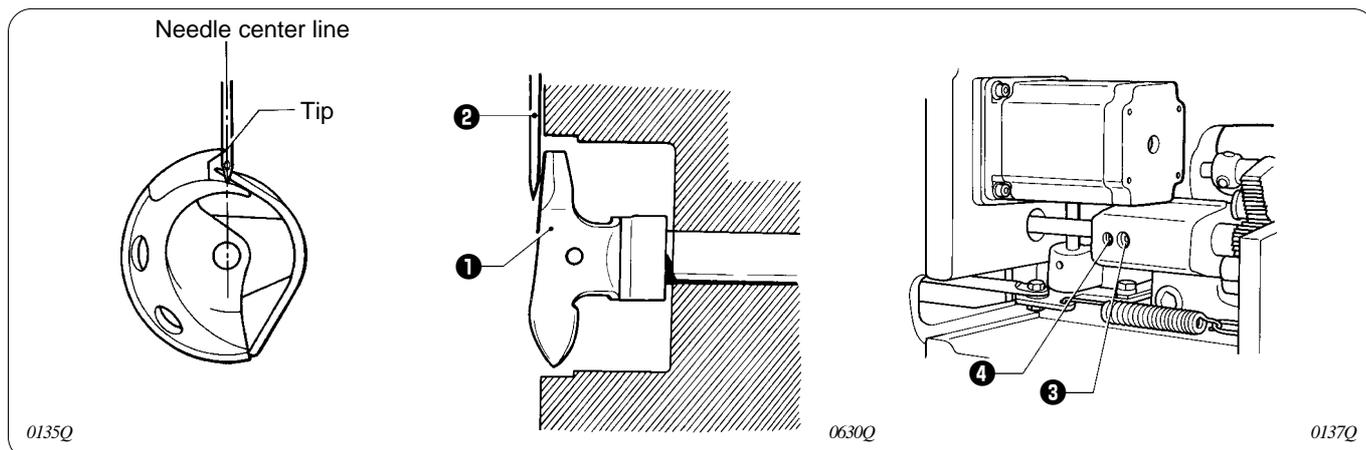
Turn the machine pulley to align the tip of the rotary hook with the needle center line. Then loosen the set screw **3** and turn the eccentric shaft **4** to adjust so that the driver needle guard **1** contacts the needle.
