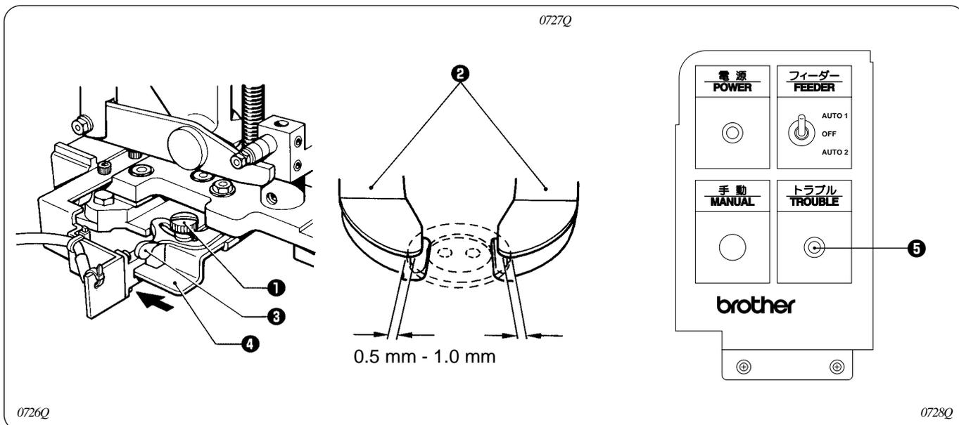
1. Loosen step screw **1** and insert a button into the button clamp **2**.
