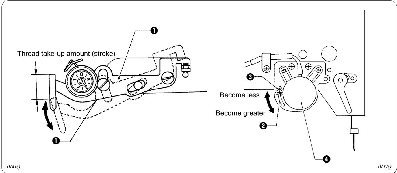
At the time of shipment from the factory, the thread take-up amount (stroke) of the thread take-up lever **1** is set to the standard setting of 5 mm. You may need to adjust this setting depending on the sewing conditions to prevent the thread from pulling out at the sewing start.
