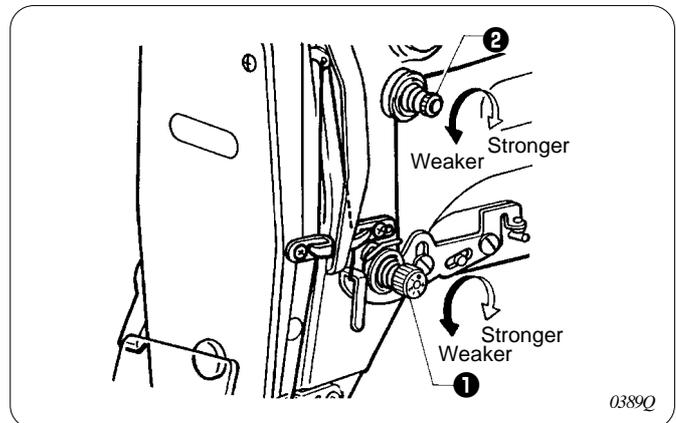
Turn the tension nut **1** (main tension) to adjust the tension as appropriate for the material being sewn. Furthermore, turn the thread nut **2** (sub-tension) to adjust the remaining length of upper thread to 35 - 40 mm when the thread take-up lever is not used.
