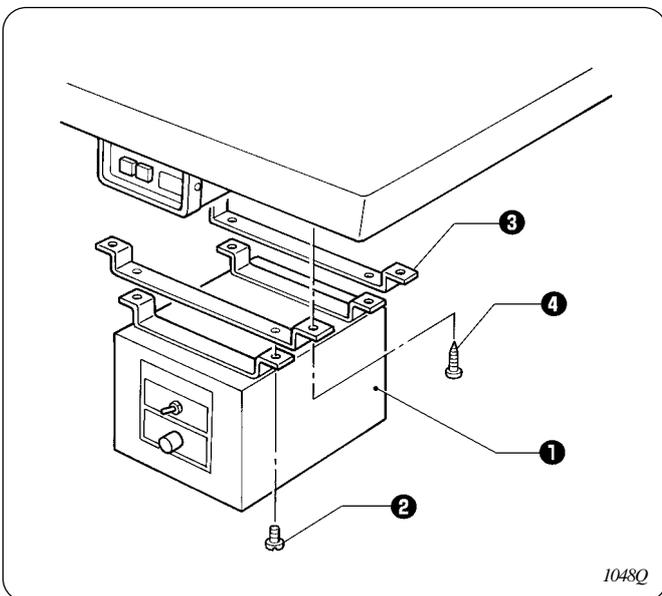
1. Mount the control box **1** to the bottom of the box stay **3** with screws **2**.
