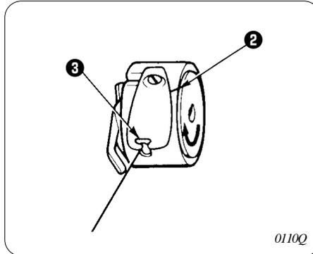
Insert a new bobbin into the bobbin case, and then pass the thread through the slot **2** and pull it out from the thread hole **3**. Check that the bobbin turns in the direction of the arrow when the thread is pulled at this time.
