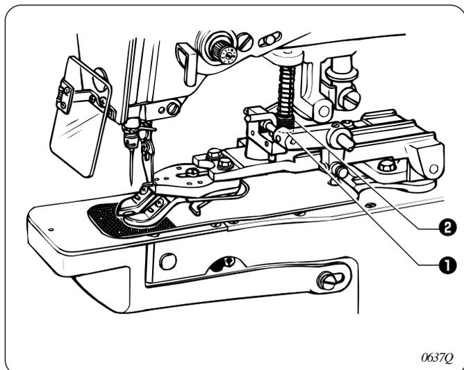
Loosen screw **1** and turn adjustment screw **2** so that clamp pressure is as light as possible but high enough so that the material will not slip when pulled lightly.
