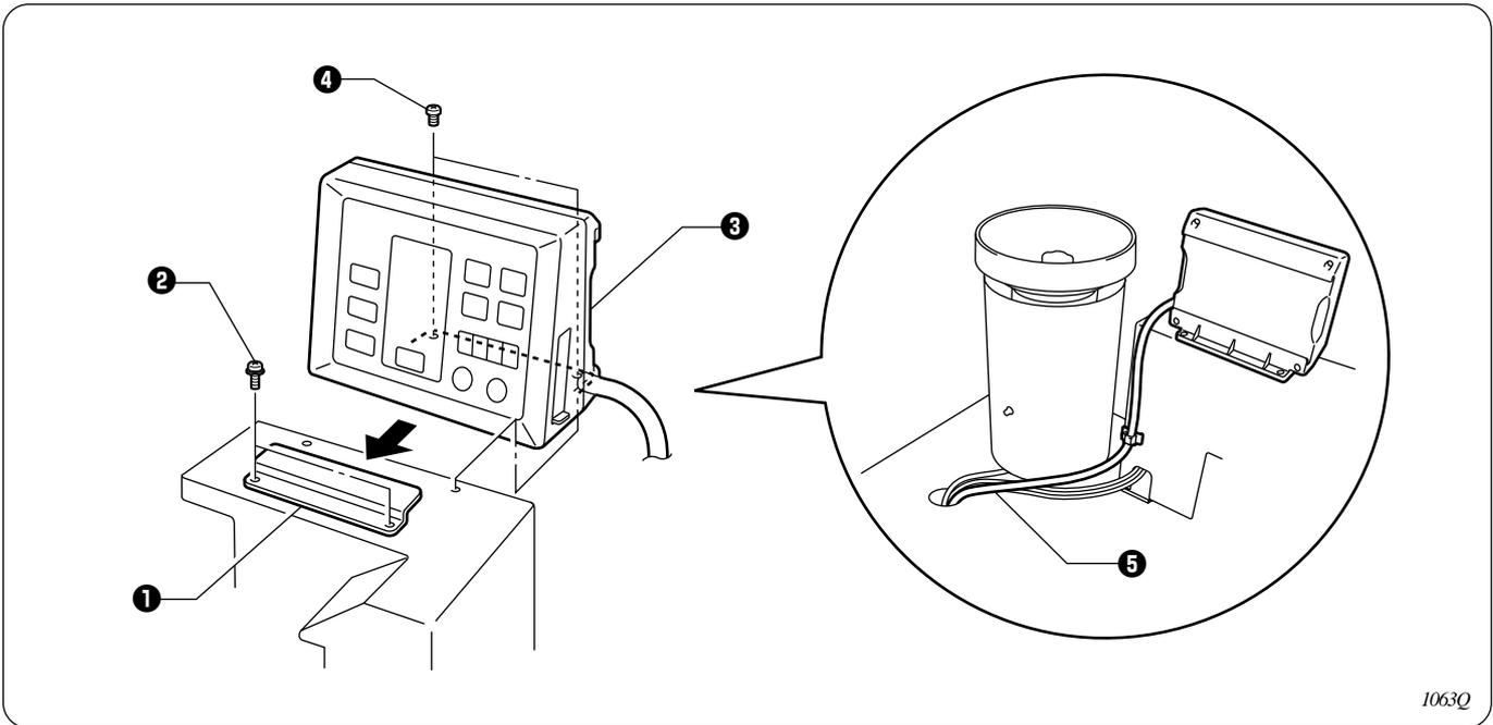
1. Install the operation panel presser plate **1** to the top of the button feeder cover with the two screws **2**.
