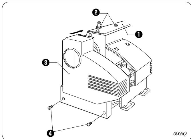
1. Loosen the two screws **2** of the upper cover **1**.
