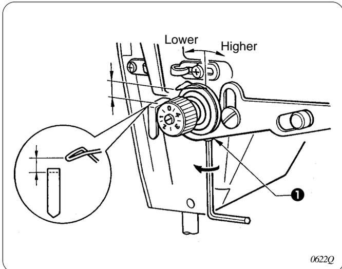
Loosen the set screw ❶ and turn the tensioner body to adjust the thread take-up spring height.
